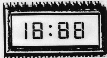
6. Dual in-line display with connectors for in-line edge plug.
