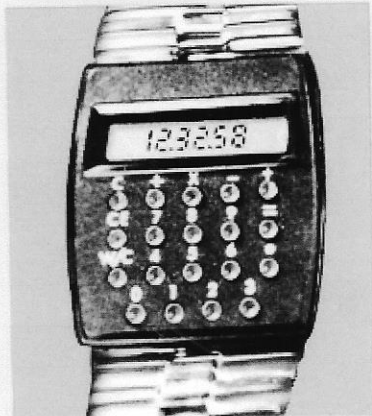
2. Wristwatch calculator with eight digit Optel display.
