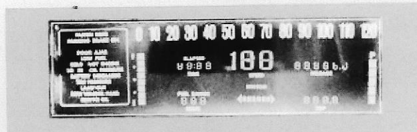
7. Automotive readout panel gives all vital driving information at a glance.
